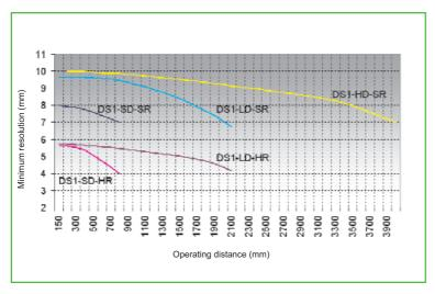
Variation of the minimum resolution according to the operating distance between the emitting and receiving units.
