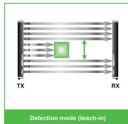
**Note:** different operating modes can be selected: absolute or relative measurement respect to a reference by means of internal dip-switches and absolute or relative detection respect to a reference by means of internal dip-switches and SET button
