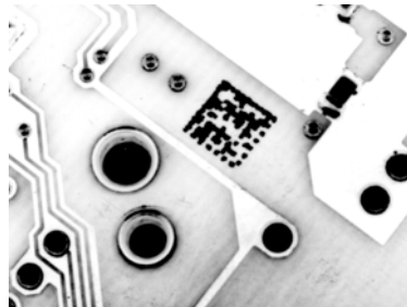
Figure 28 - DataMatrix Code Directly Marked on PCB Surface by Using Laser Etching Technology
