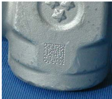
Figure 25 - Dot Matrix Code Directly Marked on Metal Surface by Using Dot Peening Technology
