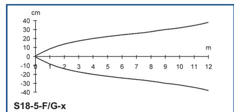
The operating distances indicate the detection distance with excess gain 2.
