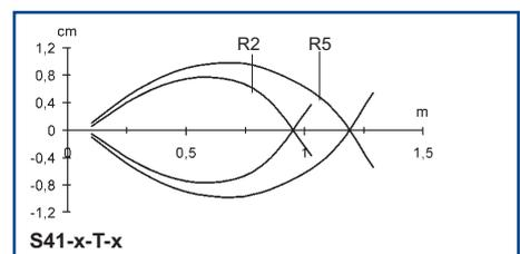
The detection diagrams indicate the typical operating distance with excess gain 1.
