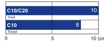
Note: the diagrams indicate the detection area typical of the axial optic versions; the maximum operating distance of the radial optic versions decreases as indicated in the tables given below
