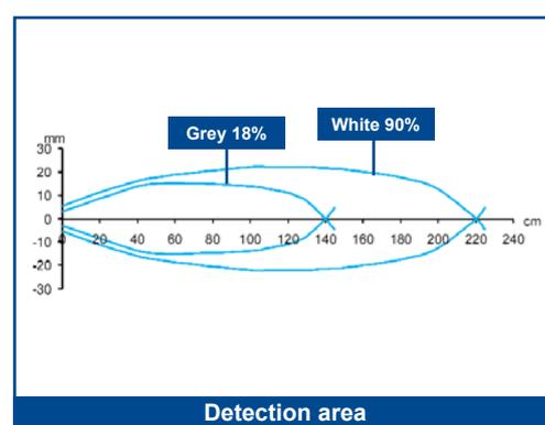
The visible red laser emission allows the accurate detection of very small objects. The sensors operate as a proximity device up to 60 cm and can be used as a contrast sensor for high contrast mark detection. The class 1 laser emission, according to EN 60825-1, guarantees maximum safety for the operators in all applications.
